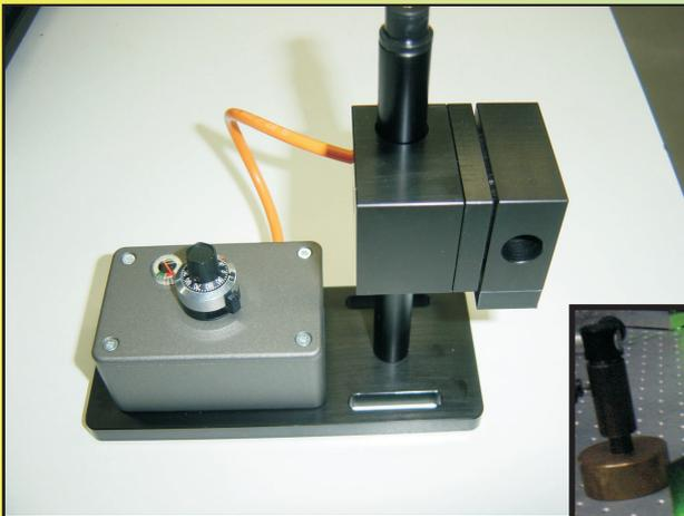
The JRS TCF-1 is optimized for 532 nm wavelength, but will give satisfactory performance for all wavelengths in the range from 490 nm to 550 nm.
